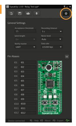
Noise level: Minimal sound volume level that can trigger a voice command recognition. Lower values require quieter pronunciation, resulting in higher noise/hiss sensitivity. On the contrary, higher level values require louder pronounciation and they are less sensitive to noise/hiss.
