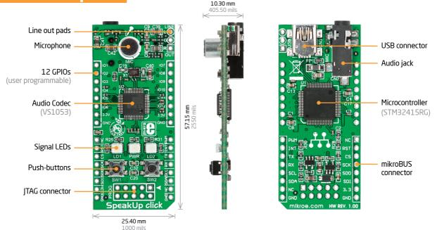
Along with its key components, the SpeakUp packs other useful bits like two buttons for recording or deleting voice commands manually, while three signal LEDs give recognition feedback and indicate power.
