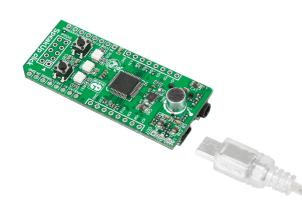
Once you connect the SpeakUp to your computer you're just a few clicks away from configuring it. The set-up process is dead simple. Launch the application, and it will lead you through the initial steps of recording and assigning commands.
