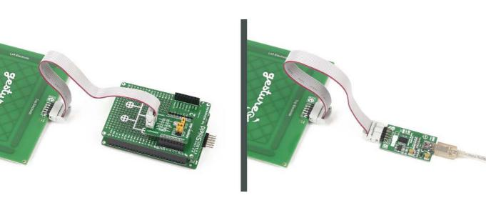
The Gesture board comes with an IDC10 connector cable. If you wish to use it for hardware prototyping, we suggest you pair it with adapter click. The other options is to develop PC applications. For that purpose we developed the Gesture USB adapter.
