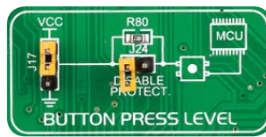
Figure 10-5: Button press level jumper (J17)
