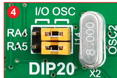
Figure 4-9: RA4 and RA5 connected to X2 quartz-crystal
