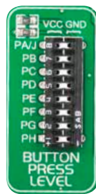
Figure 6-5: Button press level DIP switches (tri-state)
