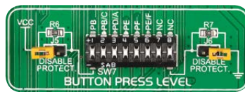
Figure 10-6: Button press level DIP switch (tri-state)
