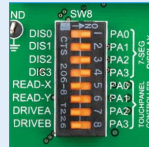
Figure 13-1: Turn on switches 1 through 4 on SW8 to enable 4-digit 7-seg display
