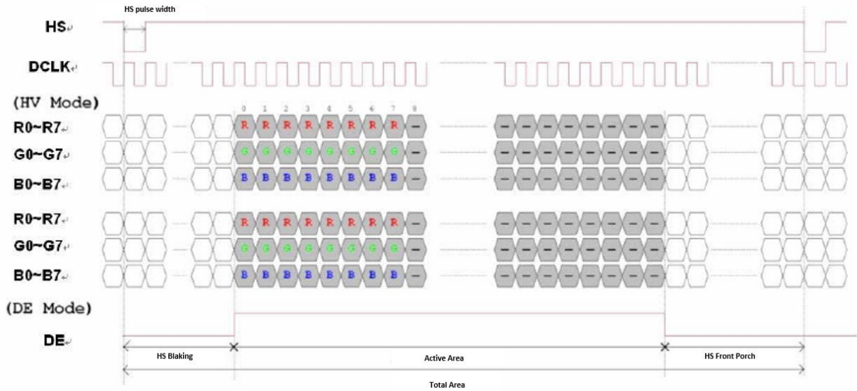
Figure 9. Horizontal input timing diagram
