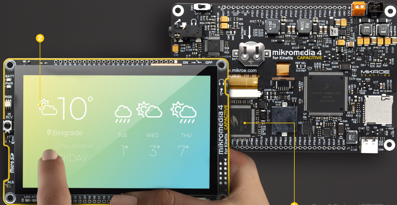
Figure 9: Display and SSD1963 view
