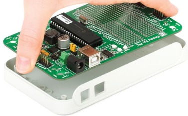
Figure 8-1: Place the board into the bottom part of the casing. Make sure that the connectors are aligned with square openings
