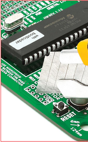
Figure 3-2: cutting copper between pads
