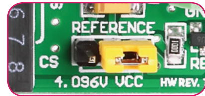
Figure 4-2: Ref. voltage is VCC
