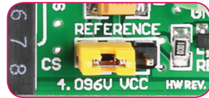
Figure 4-1: Ref. voltage is 4.096V
