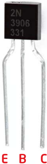
Figure A.6: 2N3906 PNP General Purpose Amplifier
