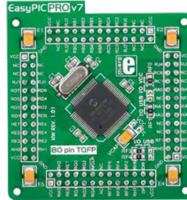
3 Figure 4-7: Standard 80-pin MCU card with PIC18F8722 .
