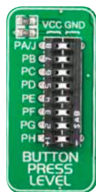
Figure 6-5: Button press level DIP switches (tri-state)
