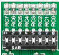
Figure 6-2: Tri-state DIP switch on PORTC
