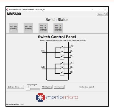
6. To connect the input ports (INA and INB) to the output ports (1A and 1B), click on either "INA 1A" switch or "INB-1B" switch, then both switches are on/off together.
