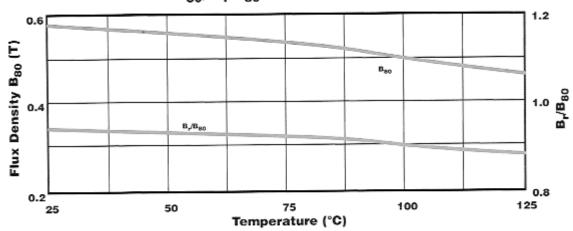
i B<sub>80</sub> = Flux Density @ 80 A/m
