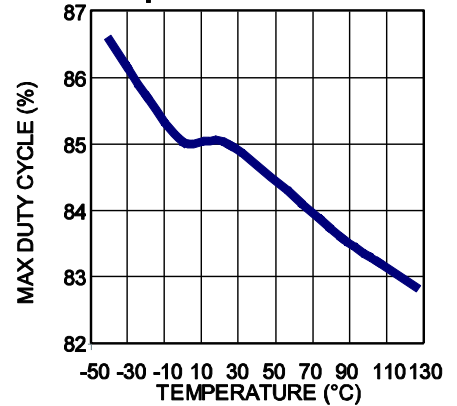
Max Duty Cycle vs. Temperature
