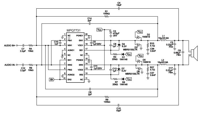
Figure 1— Mono Full Bridged Circuit
