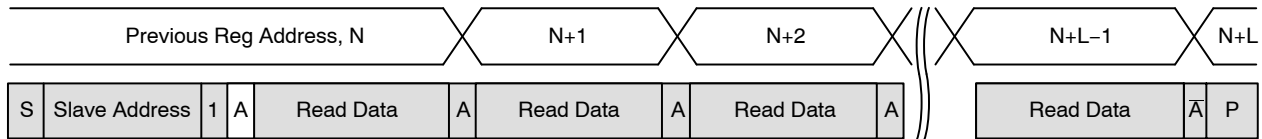
Figure 19. Sequential READ, Start from Current Location
