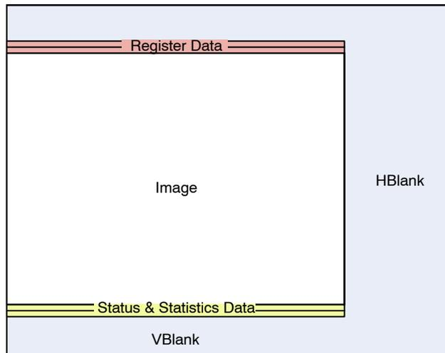
Figure 15. Frame Format with Embedded Data Lines Enabled
