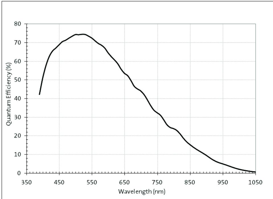
Figure 25. Estimated Quantum Efficiency – Monochrome Sensor
