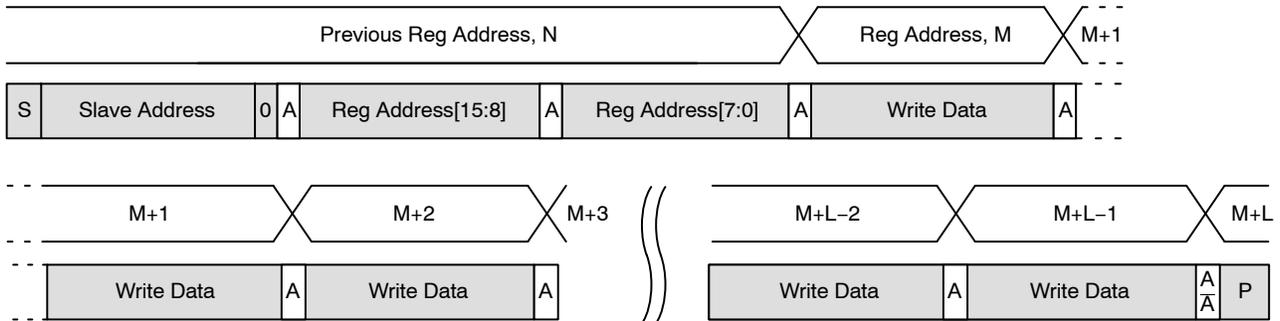
**Figure 23. Sequential WRITE, Start at Random Location**
