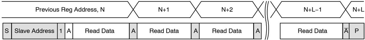
**Figure 21. Sequential READ, Start from Current Location**
