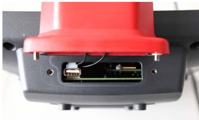
Figure 5.11: Service USB under the antenna cap
