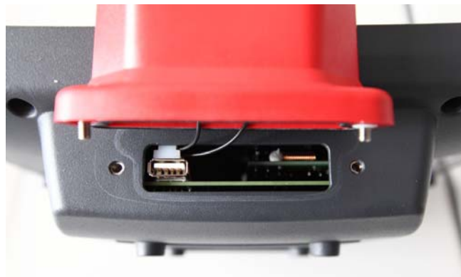
Figure 5.11: Service USB under the antenna cap
