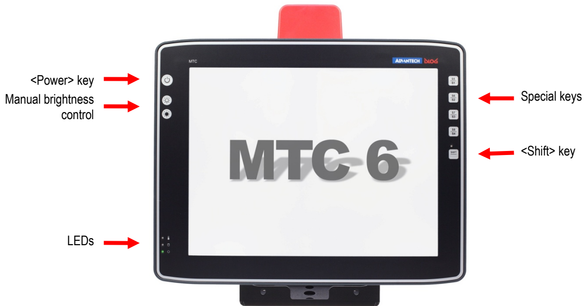
Figure 8.2: MTC 6 front keys and LEDs
