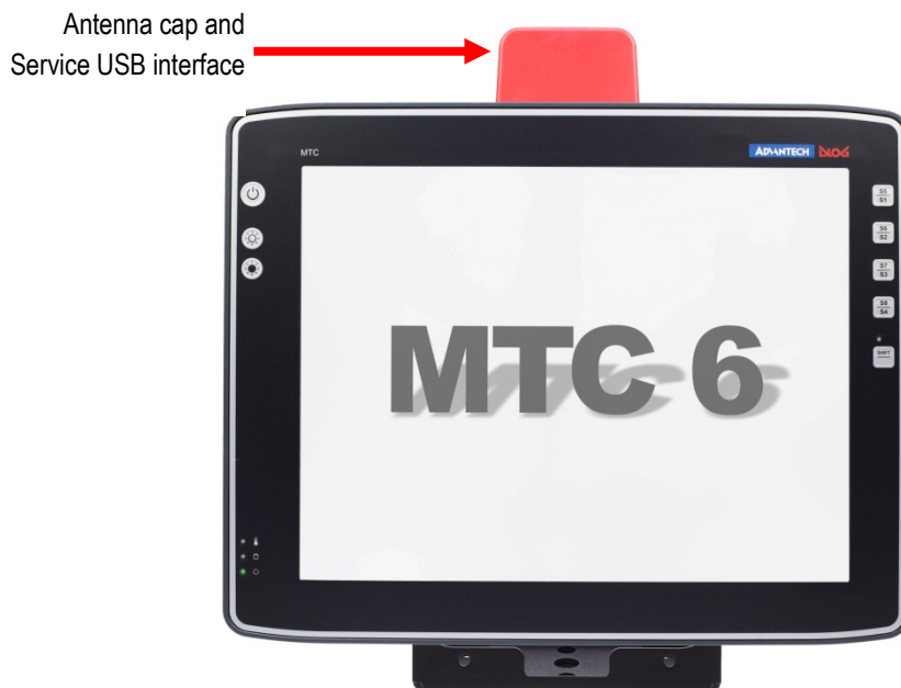
Figure 7.2: Antenna cap MTC 6
