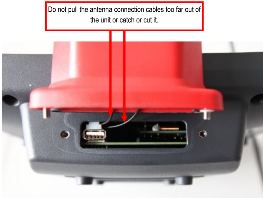
Figure 7.3: Opened antenna cap
