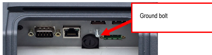
Figure 7.1: Position of the ground bolt
