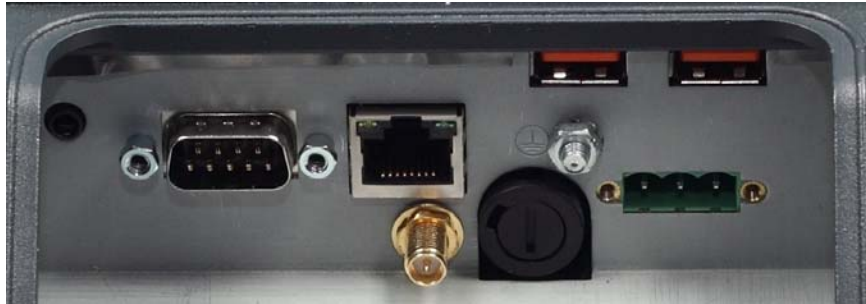
Figure 5.7: External connectors with optional ext. antenna
