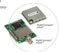
The mDot and xDot are LoRaWAN compliant,
