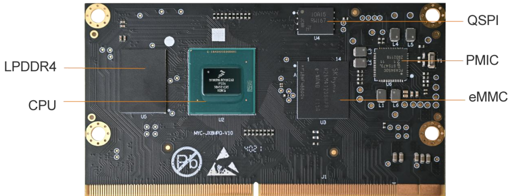
Figure 1-5 MYC-JX8MPQ CPU Module
