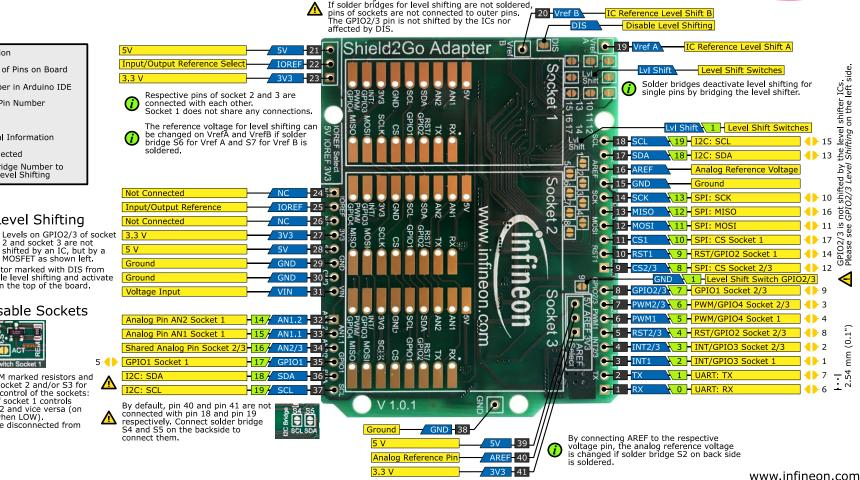
Solder bridge DIS does disable level shifter ICs if soldered.
