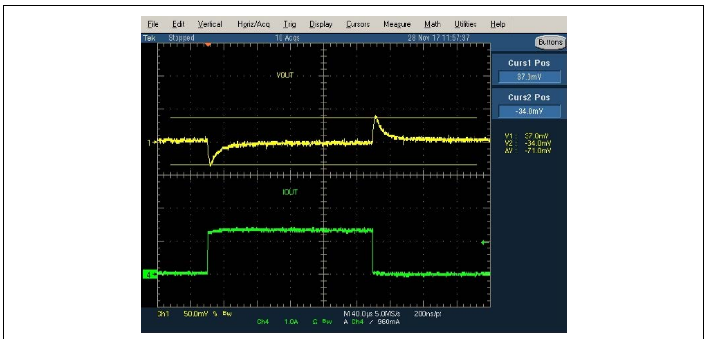
Figure 18: Damped Response without Ringing
