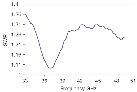
Typical SWR, 33 to 50 GHz ( 25 \pm 10^\circ\text{C} ) for N8486AQ power sensor
