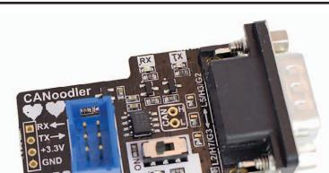
CANoodler is a simple CAN (not CAN-FD) interface, which provides logic-level 3.3V output. It's designed to be used with microcontrollers that have CAN blocks inside them, and in particular uses a pinout present on some ChipWhisperer CW308 (UFO) Target boards.
