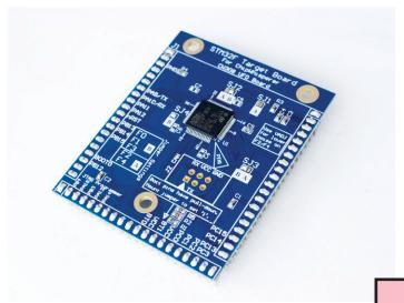
The CW308T-STM32F target series allows experiments on the popular STM32F/STM32L series of Arm devices in TQPF-64 package. This includes the STM32F0, STM32F1, STM32F2, STM32F3, STM32F4, STM32L4, and STM32L5. Devices within this family have varying core types, peripheral options, and hardware cryptographic peripheral support.
