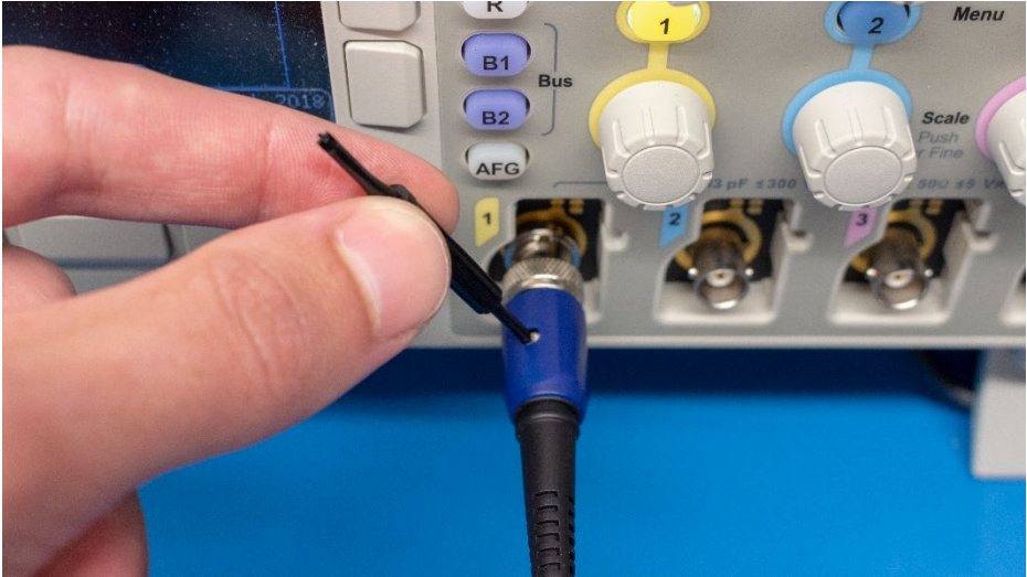
Figure 11: Tuning oscilloscope probe.
