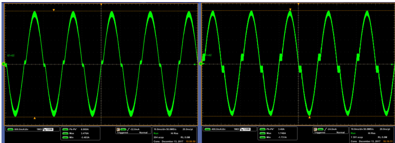
Figure 17. PFC Input Current @ 240 W Load @ 115 V AC – Left, @ 230 V AC Right
