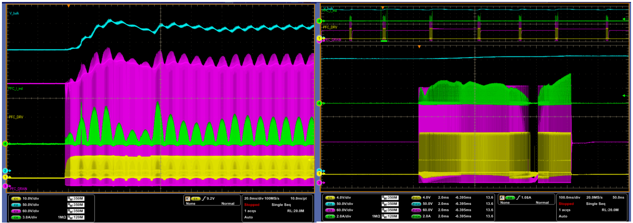
CH1 – PFC MOSFET Gate-Drive Voltage CH2 – Bulk Voltage CH3 – PFC MOSFET Drain Voltage CH4 – PFC inductor current
