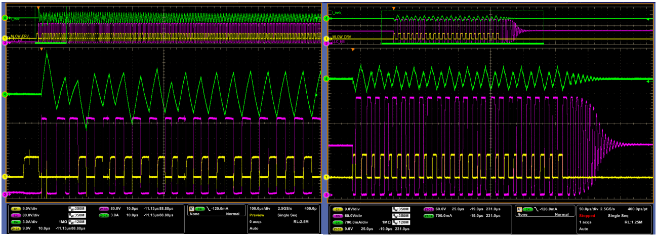
CH1 – LLC Low Side MOSFET Gate-Drive Voltage CH2 – N/A CH3 – LLC HB Node Voltage CH4 – Resonant tank current
