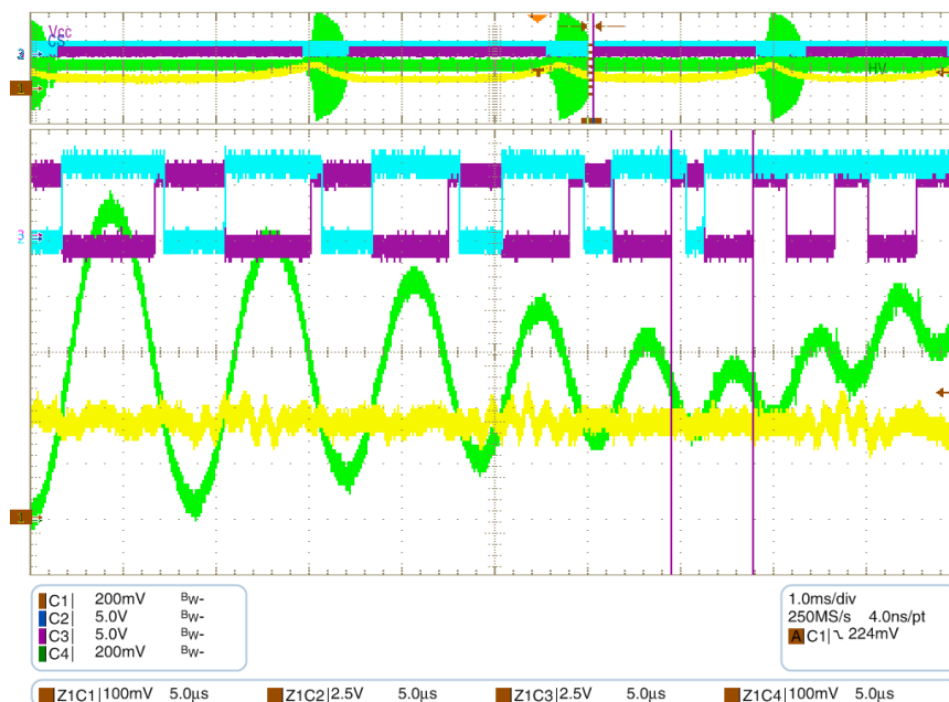
Figure 57. Mupper on-time repetition in case of transient loading when resonant capacitor imbalance occurs and on-time comparator output stays high for several periods.
