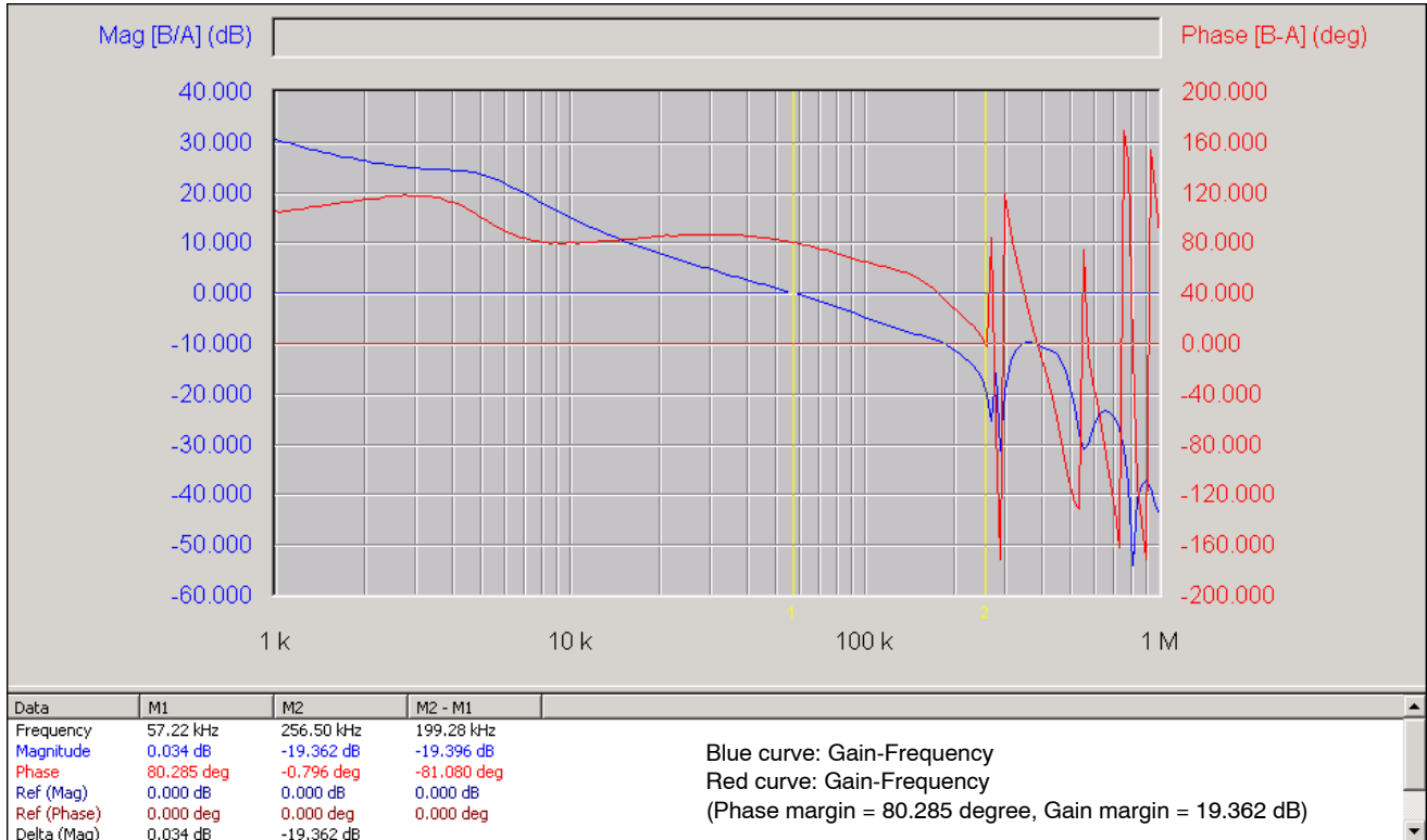
Figure 14. Closed-loop Voltage Loop-gain of the NCP1587
