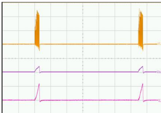
(VIN = 5 V, VOUT = 1.8 V, IOU = Current Limit, no CSS) Upper Trace: LX Pin Voltage, 5 V / div Middle Trace: Output Voltage, 2 V / div Lower Trace: Inductor Current, 2 A / div Time = 500 \mu s / div
