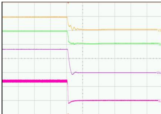
(VIN = 5 V, VOUT = 1.8 V, IOU = 3 A) Upper Trace: Input Voltage, 5 V / div Second Trace: Power Good Pin Voltage, 5 V / div Third Trace: Output Voltage, 2 V / div Lower Trace: Inductor Current, 2 A / div Time = 200 \mu s / div
