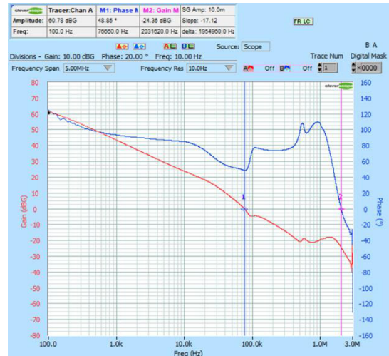
Figure 77. Bode Plot NCV6323F x LMTW11TBG L = 1.0 μH – COUT = 100 μF
