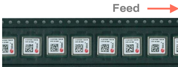
Figure 13: Orientation of NINA-W151 module on tape
