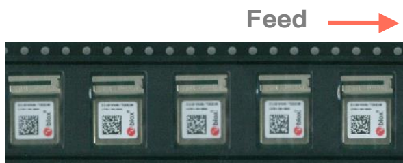
Figure 14: Orientation of NINA-W152/NINA-W156 module on tape
