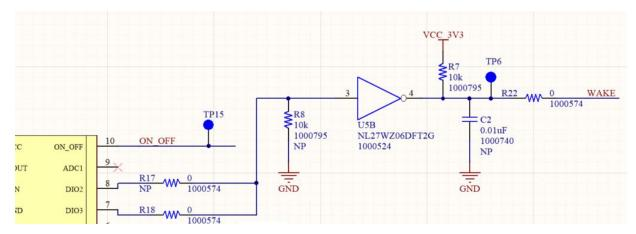
The GPIO pins on some Skywire modems may toggle while the modem is booting. If this causes an issue for the host system, the control GPIO can be changed to Skywire pin 18 by de-populating R18 and populating R17 on the adapter board.
