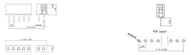
When using the recommended connector, ensure that any baseboard components placed under the Skywire (between the header connectors) are shorter than 4 mm. However, the max component height may change depending on the chosen connector.
