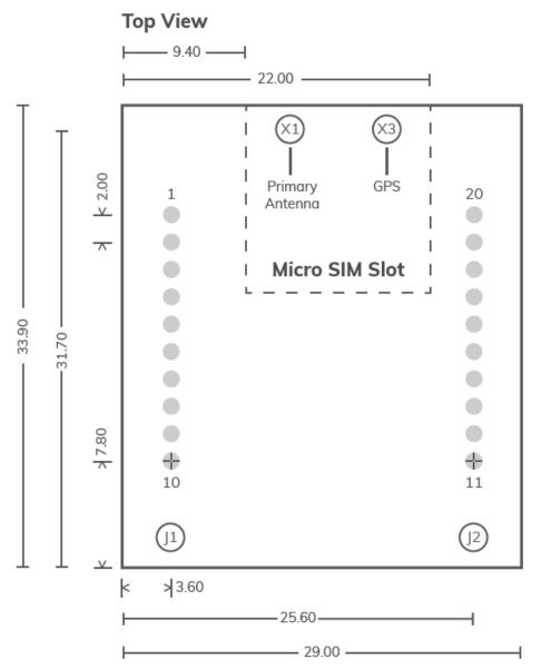
**Note:** All measurements are in millimeters. U.FL connectors X1 and X3 are on the top side of the board. Micro SIM card slot J3 is on the bottom of the board.
