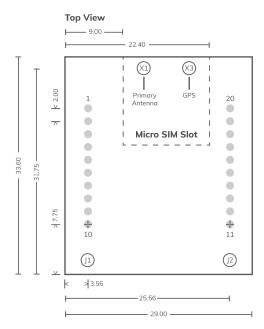
When using soldering directly to a PCB, ensure that any baseboard components placed under the Skywire (between the baseboard header pin connectors) are no taller than 0.5 mm.
