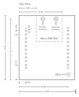
**Note:** U.FL locations are marked with circles. X1 and X2 are located on the top side of the board. X3 is the GPS antenna connector, but is not populated on the non-GPS "-NG" variants of the NL-SW-LTE-SRC7611-4 modem family. J3 is the micro SIM card slot on the bottom side of the board.
