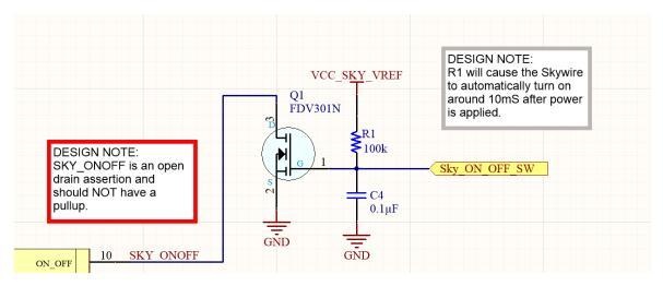
To initiate the startup procedure, tie ON\_OFF to ground for 1 < x < 2 seconds. The modem will take approximately 20 seconds to turn on and be ready for AT commands.
