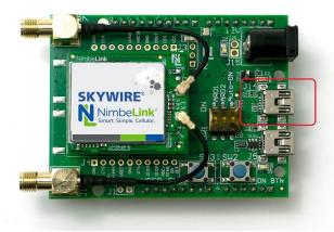
The USB to serial UART IC is an FTDI FT234XD. The FTDI drivers for the FT234XD are available on <u>FTDI's website</u>.
