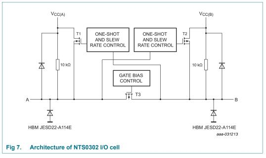
The NTS0302 is a "switch" type voltage translator using two key circuits to enable voltage translation:
