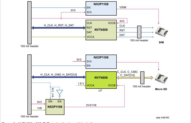
Figure 2. NVT4558-4858-EVB evaluation board block diagram
