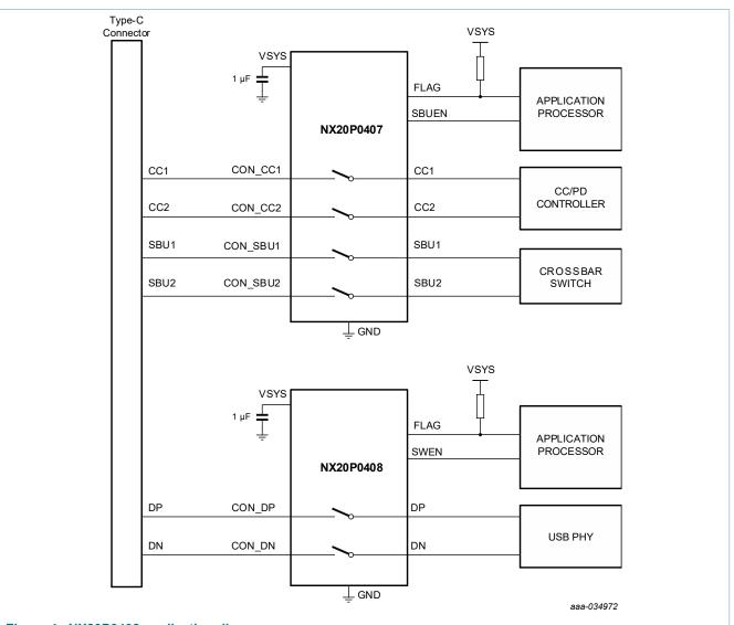
NX20P0408 is placed in front of the Type-C connector and protects D+ and D- pins in system side from 20V VBUS short, ESD and surge.
