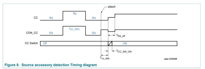
turns CC switch ON. Internal Rd is off after  $T_{Rd\_off}$ , which is for Source accessory not to lose Rd during switch transition.
