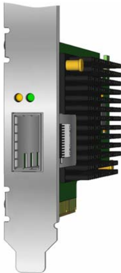
Figure 15 OCe14401B-NX/-UX Adapter LED Indicators
