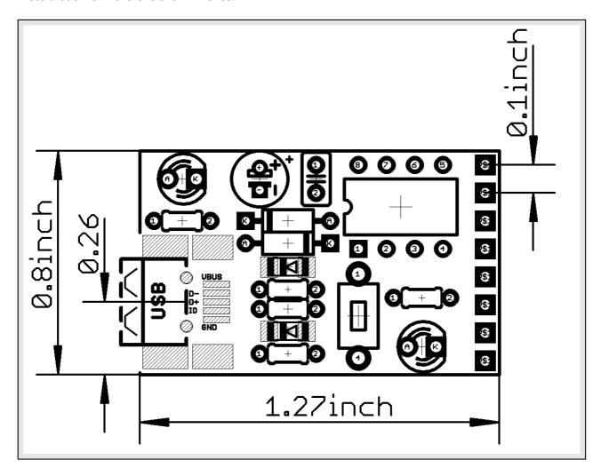
The highest element on the board is capacitor C1 with 0.5 inches of height (includes the PCB height).
