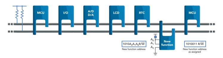
I<sup>2</sup>C-bus devices are available in a wide range of functions. Each slave device has its own I<sup>2</sup>C-bus address, selectable using address pins set high (1) or low (0). Information is transmitted byte by byte, and each byte is acknowledged by the receiver. There can be multiple devices on the same bus, and more than one IC can act as master. The master role is typically played by a microcontroller.
