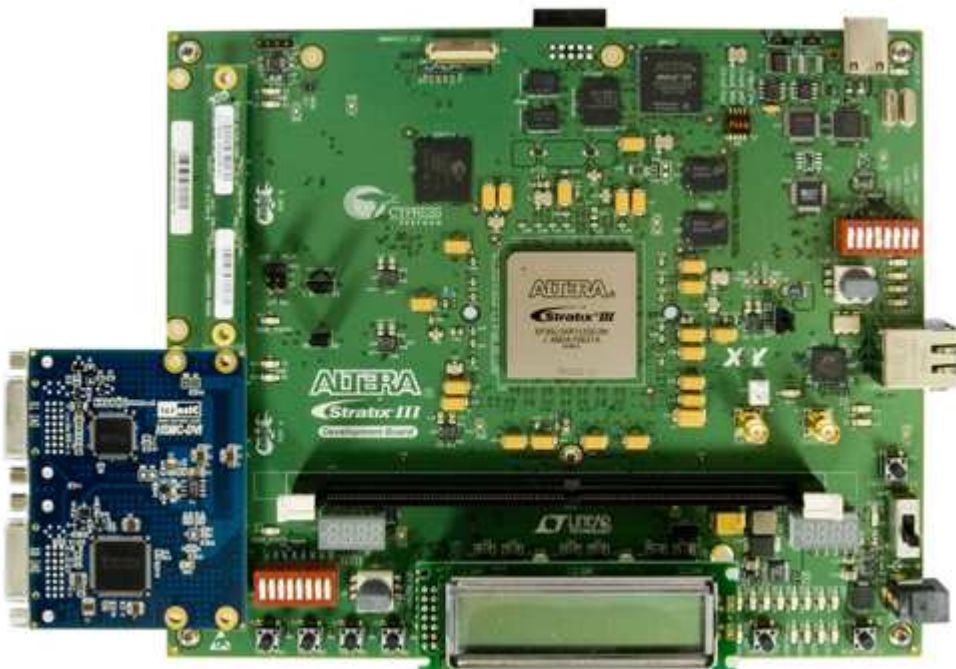
Figure 1.2.4. The HSMC-DVI board connects with Stratix III Development Board
