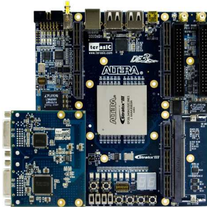
Figure 1.2.1 The HSMC-DVI board connects with DE3
